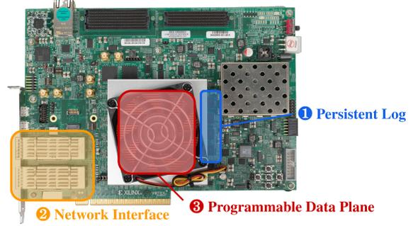
Fig. 14: FPGA platform for PMNet implementation.
